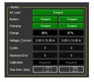
Observe the camera's internal condition and external environment. Switch off fans (Quiet Mode) to prevent vibration in microscopic applications. View battery status (if present), voltage information, fan speed and camera temperature.
